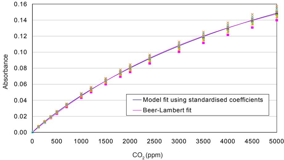
Typical response from 0 to 5000ppm CO<sub>2</sub>.
