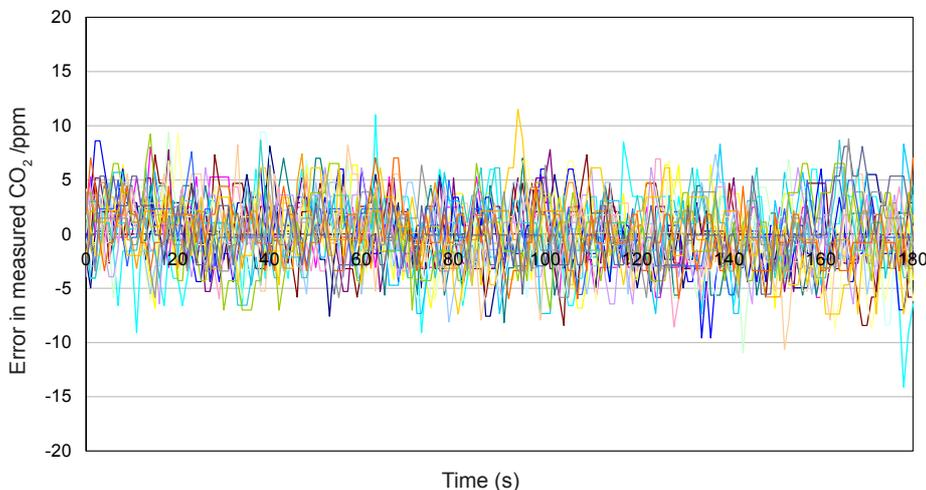
Excellent resolution and noise at 1000ppm CO<sub>2</sub> for the IRC-AT is achieved by better design, not by using more expensive components.
