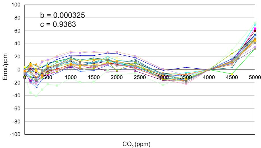
Custom linearisation is not necessary with the IRC-AT. Using universal linearisation constants, repeatability between cells is very good, allowing easy implementation.
